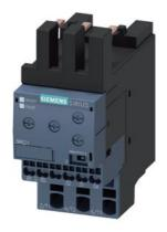
Monitoring relay, can be mounted to Contactor 3RT2, Size S0 basic, analog adjustment Apparent current monitoring 4...40 A, 50...60 Hz, 2-phase Supply 24-240 V AC/DC 1 change-over contact Monitoring for Current overshoot and undershoot Phase failure, Cable break with or without fault buffer ON delay 0-60 s Noise pulse suppression 0-30 s Switching hysteresis 6% spring-type connection system
