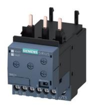
Monitoring relay, can be mounted to Contactor 3RT2, Size S0 basic, analog adjustment Apparent current monitoring 4...40 A, 50...60 Hz, 2-phase Supply 24-240 V AC/DC 1 change-over contact Monitoring for Current overshoot and undershoot Phase failure, Cable break with or without fault buffer ON delay 0-60 s Noise pulse suppression 0-30 s Switching hysteresis 6% Screw connection system
