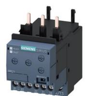
Monitoring relay, can be mounted to Contactor 3RT2, Size S0 basic, analog adjustment Apparent current monitoring 4...40 A, 50...60 Hz, 2-phase Supply 24 V AC/DC 1 change-over contact Monitoring for Current overshoot and undershoot Phase failure, Cable break with or without fault buffer ON delay 0-60 s Noise pulse suppression 0-30 s Switching hysteresis 6% Screw connection system
