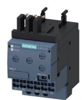
Monitoring relay, can be mounted to Contactor 3RT2, Size S00 basic, analog adjustment Apparent current monitoring 1.6-16 A, 20-400 Hz, 2-phase Supply 24 V AC/DC 1 change-over contact Monitoring for Current overshoot and undershoot Phase failure, Cable break with or without fault buffer ON delay 0-60 s Noise pulse suppression 0-30 s Switching hysteresis 6% spring-type connection system
