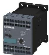
Timing relay, electronic slow-operating 1 change-over contact 24 V AC/DC, 200 to 127 V AC at 50/60 Hz AC 0.05 s to 100 h Overall width 45 mm Spring-type terminal
