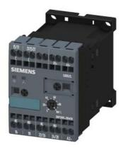
Timing relay, electronic Multifunction, 16 functions 2 change-over contacts 24 to 240 V AC/DC at 50/60 Hz AC 0.05 s to 100 h Overall width 45 mm Spring-type terminal
