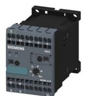
Timing relay, electronic Multifunction, 8 functions 1 change-over contact 24 V AC/DC, 200 to 240 V AC at 50/60 Hz AC 0.05 s to 100 h Overall width 45 mm Spring-type terminal
