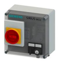
SIRIUS MCU motor starter Enclosure degree of protection IP55 plastic Communication without electromechanically switching short-circuit protection with circuit breaker Reversing starter Brake without performance class 3.2 A Motor circuit breaker with bi-metal thermal Manual operation latching Connection power M screw connection Electrical wholesale version
