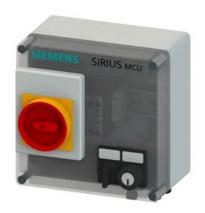
SIRIUS MCU motor starter Enclosure degree of protection IP55 plastic Communication without electromechanically switching Short-circuit protection with circuit breaker Reversing starter Brake without Performance class 1.6 A Motor circuit breaker with bi-metal thermal Manual operation latching Connection power M screw connection Electrical wholesale version
