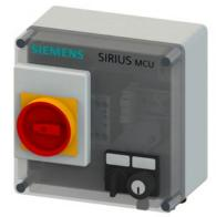
SIRIUS MCU motor starter Enclosure degree of protection IP55 plastic Communication without electromechanically switching Short-circuit protection with circuit breaker DOL starter Brake without Performance class 1.6 A Motor circuit breaker with bi-metal thermal Manual operation latching Connection power M screw connection Electrical wholesale version
