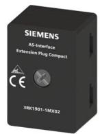
AS-i Extension Plug Compact Doubling of the cable length to 200 m per AS-Interface segment Degree of protection IP67 Connection directly to AS-i Flat ribbon cable
