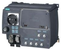
SIRIUS motor starter M200D Technology module Reversing starter Electronic switching AC-3, 5.5 kW / 400 V 1.5 A...12.00 A Electronic overload protection Thermistor: THERMOCLICK / PTC with brake contact 400 V AC 4 DI / 2 DO Han Q4/2 - Han Q8/0 with manual on-site operation and key-operated switch via communication module 3RK1305\* can be used on PROFIBUS or PROFINET
