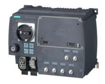
SIRIUS motor starter M200D Technology module DOL starter Electronic switching AC-3, 5.5 kW / 400 V 1.5 A...12.00 A Electronic overload protection Thermistor: THERMOCLICK / PTC with brake contact 180 V DC 4 DI / 2 DO Han Q4/2 - Han Q8/0 with manual on-site operation and key-operated switch via communication module 3RK1305\* can be used on PROFIBUS or PROFINET
