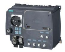
SIRIUS motor starter M200D Technology module DOL starter Electronic switching AC-3, 5.5 kW / 400 V 1.5 A...12.00 A Electronic overload protection Thermistor: THERMOCLICK / PTC with brake contact 400 V AC 4 DI / 2 DO Han Q4/2 - Han Q8/0 with manual on-site operation and key-operated switch via communication module 3RK1305\* can be used on PROFIBUS or PROFINET
