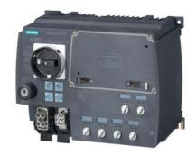
SIRIUS motor starter M200D Technology module DOL starter Electronic switching AC-3, 5.5 kW / 400 V 1.5 A...12.00 A Electronic overload protection Thermistor: THERMOCLICK / PTC without brake contact 4 DI / 2 DO Han Q4/2 - Han Q8/0 with manual on-site operation and key-operated switch via communication module 3RK1305\* can be used on PROFIBUS or PROFINET
