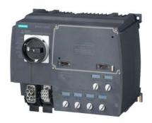
SIRIUS motor starter M200D Technology module Reversing starter Electronic switching AC-3, 5.5 kW / 400 V 1.5 A...12.00 A Electronic overload protection Thermistor: THERMOCLICK / PTC with brake contact 180 V DC 4 DI / 2 DO Han Q4/2 - Han Q8/0 via communication module 3RK1305\* can be used on PROFIBUS or PROFINET
