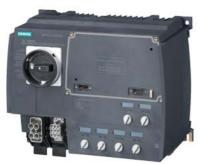
SIRIUS motor starter M200D Technology module Reversing starter Electronic switching AC-3, 5.5 kW / 400 V 1.5 A...12.00 A Electronic overload protection Thermistor: THERMOCLICK / PTC without brake contact 4 DI / 2 DO Han Q4/2 - Han Q8/0 via communication module 3RK1305\* can be used on PROFIBUS or PROFINET
