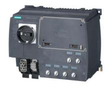
SIRIUS motor starter M200D Technology module DOL starter Electronic switching AC-3, 5.5 kW / 400 V 1.5 A...12.00 A Electronic overload protection Thermistor: THERMOCLICK / PTC with brake contact 180 V DC 4 DI / 2 DO Han Q4/2 - Han Q8/0 via communication module 3RK1305\* can be used on PROFIBUS or PROFINET
