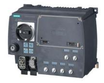
SIRIUS motor starter M200D Technology module Reversing starter Mechanical switching AC-3, 5.5 kW / 400 V 1.5 A...12.00 A Electronic overload protection Thermistor: THERMOCLICK / PTC with brake contact 180 V DC 4 DI / 2 DO Han Q4/2 - Han Q8/0 with manual on-site operation and key-operated switch via communication module 3RK1305\* can be used on PROFIBUS or PROFINET
