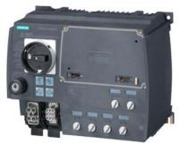
SIRIUS motor starter M200D Technology module Reversing starter Mechanical switching AC-3, 5.5 kW / 400 V 1.5 A...12.00 A Electronic overload protection Thermistor: THERMOCLICK / PTC with brake contact 400 V AC 4 DI / 2 DO Han Q4/2 - Han Q8/0 with manual on-site operation and key-operated switch via communication module 3RK1305\* can be used on PROFIBUS or PROFINET
