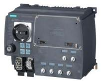
SIRIUS motor starter M200D Technology module Reversing starter Mechanical switching AC-3, 5.5 kW / 400 V 1.5 A...12.00 A Electronic overload protection Thermistor: THERMOCLICK / PTC without brake contact 4 DI / 2 DO Han Q4/2 - Han Q8/0 with manual on-site operation and key-operated switch via communication module 3RK1305\* can be used on PROFIBUS or PROFINET
