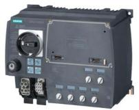
SIRIUS motor starter M200D Technology module DOL starter Mechanical switching AC-3, 5.5 kW / 400 V 1.5 A...12.00 A Electronic overload protection Thermistor: THERMOCLICK / PTC with brake contact 400 V AC 4 DI / 2 DO Han Q4/2 - Han Q8/0 with manual on-site operation and key-operated switch via communication module 3RK1305\* can be used on PROFIBUS or PROFINET
