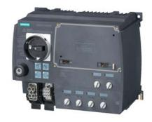
SIRIUS motor starter M200D Technology module DOL starter Mechanical switching AC-3, 5.5 kW / 400 V 1.5 A...12.00 A Electronic overload protection Thermistor: THERMOCLICK / PTC without brake contact 4 DI / 2 DO Han Q4/2 - Han Q8/0 with manual on-site operation and key-operated switch via communication module 3RK1305\* can be used on PROFIBUS or PROFINET
