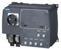
SIRIUS motor starter M200D Technology module Reversing starter Mechanical switching AC-3, 5.5 kW / 400 V 1.5 A...12.00 A Electronic overload protection Thermistor: THERMOCLICK / PTC with brake contact 180 V DC 4 DI / 2 DO Han Q4/2 - Han Q8/0 via communication module 3RK1305\* can be used on PROFIBUS or PROFINET
