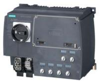
SIRIUS motor starter M200D Technology module DOL starter Mechanical switching AC-3, 5.5 kW / 400 V 1.5 A...12.00 A Electronic overload protection Thermistor: THERMOCLICK / PTC with brake contact 400 V AC 4 DI / 2 DO Han Q4/2 - Han Q8/0 via communication module 3RK1305\* can be used on PROFIBUS or PROFINET
