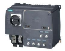
SIRIUS motor starter M200D Technology module DOL starter Mechanical switching AC-3, 5.5 kW / 400 V 1.5 A...12.00 A Electronic overload protection Thermistor: THERMOCLICK / PTC without brake contact 4 DI / 2 DO Han Q4/2 - Han Q8/0 via communication module 3RK1305\* can be used on PROFIBUS or PROFINET
