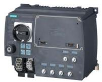
SIRIUS motor starter M200D Technology module Reversing starter Electronic switching AC-3, 0.75KW / 400 V 0.15 A...2.00 A Electronic overload protection Thermistor: THERMOCLICK / PTC without brake contact 4 DI / 2 DO Han Q4/2 - Han Q8/0 with manual on-site operation and key-operated switch via communication module 3RK1305\* can be used on PROFIBUS or PROFINET
