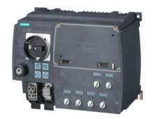
SIRIUS motor starter M200D Technology module DOL starter Electronic switching AC-3, 0.75KW / 400 V 0.15 A...2.00 A Electronic overload protection Thermistor: THERMOCLICK / PTC without brake contact 4 DI / 2 DO Han Q4/2 - Han Q8/0 with manual on-site operation and key-operated switch via communication module 3RK1305\* can be used on PROFIBUS or PROFINET
