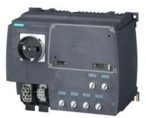
SIRIUS motor starter M200D Technology module Reversing starter Electronic switching AC-3, 0.75KW / 400 V 0.15 A...2.00 A Electronic overload protection Thermistor: THERMOCLICK / PTC without brake contact 4 DI / 2 DO Han Q4/2 - Han Q8/0 via communication module 3RK1305\* can be used on PROFIBUS or PROFINET
