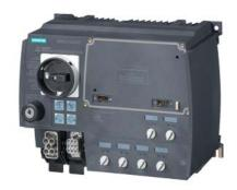
SIRIUS motor starter M200D Technology module Reversing starter Mechanical switching AC-3, 0.75KW / 400 V 0.15 A...2.00 A Electronic overload protection Thermistor: THERMOCLICK / PTC with brake contact 400 V AC 4 DI / 2 DO Han Q4/2 - Han Q8/0 with manual on-site operation and key-operated switch via communication module 3RK1305\* can be used on PROFIBUS or PROFINET
