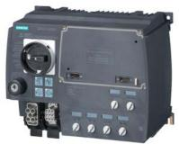
SIRIUS motor starter M200D Technology module DOL starter Mechanical switching AC-3, 0.75KW / 400 V 0.15 A...2.00 A Electronic overload protection Thermistor: THERMOCLICK / PTC without brake contact 4 DI / 2 DO Han Q4/2 - Han Q8/0 with manual on-site operation and key-operated switch via communication module 3RK1305\* can be used on PROFIBUS or PROFINET
