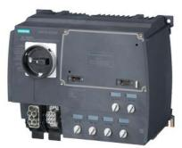
SIRIUS motor starter M200D Technology module Reversing starter Mechanical switching AC-3, 0.75KW / 400 V 0.15 A...2.00 A Electronic overload protection Thermistor: THERMOCLICK / PTC without brake contact 4 DI / 2 DO Han Q4/2 - Han Q8/0 via communication module 3RK1305\* can be used on PROFIBUS or PROFINET
