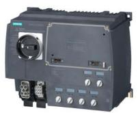
SIRIUS motor starter M200D Technology module DOL starter Mechanical switching AC-3, 0.75KW / 400 V 0.15 A...2.00 A Electronic overload protection Thermistor: THERMOCLICK / PTC with brake contact 180 V DC 4 DI / 2 DO Han Q4/2 - Han Q8/0 via communication module 3RK1305\* can be used on PROFIBUS or PROFINET
