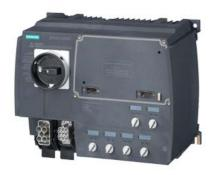
SIRIUS motor starter M200D Technology module DOL starter Mechanical switching AC-3, 0.75KW / 400 V 0.15 A...2.00 A Electronic overload protection Thermistor: THERMOCLICK / PTC with brake contact 400 V AC 4 DI / 2 DO Han Q4/2 - Han Q8/0 via communication module 3RK1305\* can be used on PROFIBUS or PROFINET
