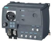
SIRIUS motor starter M200D AS-i Communication: AS-Interface Reversing starter standard Electronic switching AC-3, 5.5 kW / 400 V 1.5 A...12.00 A Electronic overload protection Thermistor: THERMOCLICK / PTC with brake contact 400 V AC 4 DI / 1 DO AS-i Han Q4/2 - Han Q8/0 with manual on-site operation and key-operated switch
