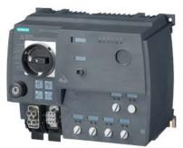
SIRIUS motor starter M200D AS-i Communication: AS-Interface DOL starter Standard Electronic switching AC-3, 5.5 kW / 400 V 1.5 A...12.00 A Electronic overload protection Thermistor: THERMOCLICK / PTC with brake contact 180 V DC 4 DI / 1 DO AS-i Han Q4/2 - Han Q8/0 with manual on-site operation and key-operated switch
