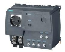
SIRIUS motor starter M200D AS-i Communication: AS-Interface DOL starter Standard Electronic switching AC-3, 5.5 kW / 400 V 1.5 A...12.00 A Electronic overload protection Thermistor: THERMOCLICK / PTC with brake contact 180 V DC 4 DI / 1 DO AS-i Han Q4/2 - Han Q8/0
