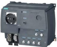
SIRIUS motor starter M200D AS-i Communication: AS-Interface DOL starter Standard Electronic switching AC-3, 5.5 kW / 400 V 1.5 A...12.00 A Electronic overload protection Thermistor: THERMOCLICK / PTC without brake contact 4 DI / 1 DO AS-i Han Q4/2 - Han Q8/0
