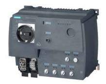
SIRIUS motor starter M200D AS-i Communication: AS-Interface DOL starter Standard Mechanical switching AC-3, 5.5 kW / 400 V 1.5 A...12.00 A Electronic overload protection Thermistor: THERMOCLICK / PTC with brake contact 180 V DC 4 DI / 1 DO AS-i Han Q4/2 - Han Q8/0
