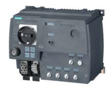
SIRIUS motor starter M200D AS-i Communication: AS-Interface Reversing starter standard Electronic switching AC-3, 0.75KW / 400 V 0.15 A...2.00 A Electronic overload protection Thermistor: THERMOCLICK / PTC with brake contact 400 V AC 4 DI / 1 DO AS-i Han Q4/2 - Han Q8/0 with manual on-site operation and keyoperated switch
