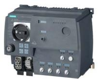
SIRIUS motor starter M200D AS-i Communication: AS-Interface DOL starter Standard Electronic switching AC-3, 0.75KW / 400 V 0.15 A...2.00 A Electronic overload protection Thermistor: THERMOCLICK / PTC without brake contact 4 DI / 1 DO AS-i Han Q4/2 - Han Q8/0 with manual on-site operation and key-operated switch
