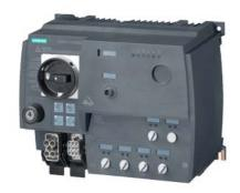
SIRIUS motor starter M200D AS-i Communication: AS-Interface Reversing starter standard Mechanical switching AC-3, 0.75KW / 400 V 0.15 A...2.00 A Electronic overload protection Thermistor: THERMOCLICK / PTC with brake contact 180 V DC 4 DI / 1 DO AS-i Han Q4/2 - Han Q8/0 with manual on-site operation and keyoperated switch
