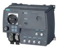
SIRIUS motor starter M200D AS-i Communication: AS-Interface Reversing starter standard Mechanical switching AC-3, 0.75KW / 400 V 0.15 A...2.00 A Electronic overload protection Thermistor: THERMOCLICK / PTC with brake contact 400 V AC 4 DI / 1 DO AS-i Han Q4/2 - Han Q8/0 with manual on-site operation and keyoperated switch
