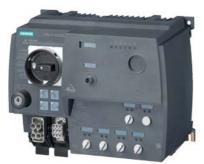
SIRIUS motor starter M200D AS-i Communication: AS-Interface DOL starter Standard Mechanical switching AC-3, 0.75KW / 400 V 0.15 A...2.00 A Electronic overload protection Thermistor: THERMOCLICK / PTC with brake contact 180 V DC 4 DI / 1 DO AS-i Han Q4/2 - Han Q8/0 with manual on-site operation and keyoperated switch
