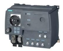
SIRIUS motor starter M200D AS-i Communication: AS-Interface DOL starter Standard Mechanical switching AC-3, 0.75KW / 400 V 0.15 A...2.00 A Electronic overload protection Thermistor: THERMOCLICK / PTC without brake contact 4 DI / 1 DO AS-i Han Q4/2 - Han Q8/0 with manual on-site operation and key-operated switch
