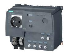
SIRIUS motor starter M200D AS-i Communication: AS-Interface DOL starter Standard Mechanical switching AC-3, 0.75KW / 400 V 0.15 A...2.00 A Electronic overload protection Thermistor: THERMOCLICK / PTC with brake contact 180 V DC 4 DI / 1 DO AS-i Han Q4/2 - Han Q8/0
