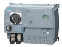
SIRIUS motor starter M200D AS-i Communication: AS-Interface Reversing starter Basic Electronic switching AC-3, 4 kW / 400 V 1.5 A...9.00 A Electronic overload protection Thermistor: THERMOCLICK / PTC without brake contact 2DI AS-i + 2DI / 1DO on device Han Q4/2 - Han Q8/0 with manual on-site operation and keyoperated switch
