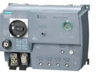
SIRIUS motor starter M200D AS-i Communication: AS-Interface DOL starter Basic Electronic switching AC-3, 4 kW / 400 V 1.5 A...9.00 A Electronic overload protection Thermistor: THERMOCLICK / PTC with brake contact 180 V DC 2DI AS-i + 2DI / 1DO on device Han Q4/2 - Han Q8/0 with manual on-site operation and key-operated switch
