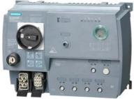
SIRIUS motor starter M200D AS-i Communication: AS-Interface DOL starter Basic Electronic switching AC-3, 4 kW / 400 V 1.5 A...9.00 A Electronic overload protection Thermistor: THERMOCLICK / PTC without brake contact 2DI AS-i + 2DI / 1DO on device Han Q4/2 - Han Q8/0 with manual on-site operation and key-operated switch
