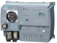
SIRIUS motor starter M200D AS-i Communication: AS-Interface DOL starter Basic Mechanical switching AC-3, 5.5 kW / 400 V 1.5 A...12.00 A Electronic overload protection Thermistor: THERMOCLICK / PTC with brake contact 180 V DC 2DI AS-i + 2DI / 1DO on device Han Q4/2 - Han Q8/0 with manual on-site operation and key-operated switch
